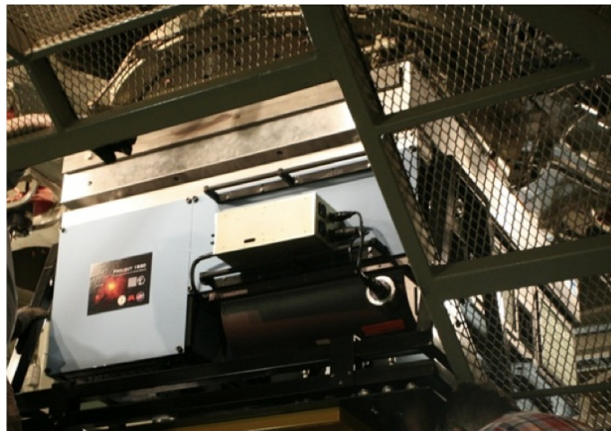
Figure 1. The PALMAO system and Project 1640 coronagraphic integral field spectrograph mounted at the Cassegrain focus of the Palomar Hale telescope.
