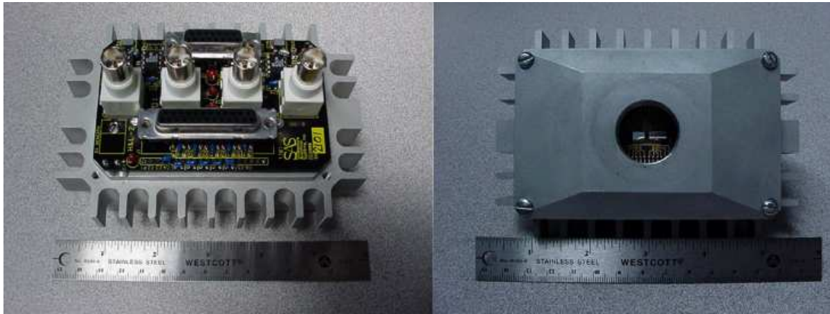
Figure 6. SciMeasure's new remote CCD camera head. This head may be located up to 8m away from the controller box in Figure 5, without measurable increase in camera noise.
