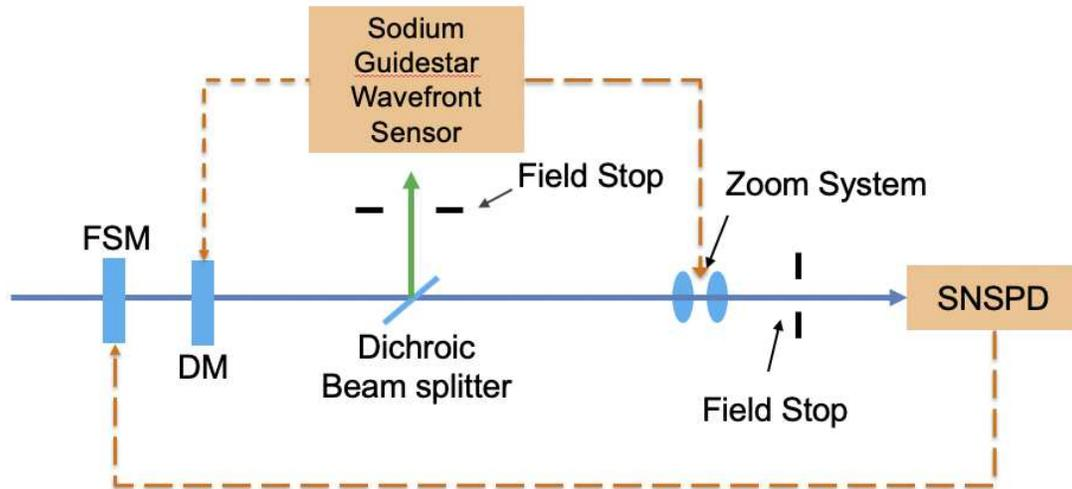
Figure 2. This is a block diagram of the proposed AO concept for communicating with spacecraft in Deep Space. The blue arrow is the light path of the system (with all the FSM and DM being depicted as transmissive to simplify the diagram.) The dashed lines are control signals from sensors to active elements.
