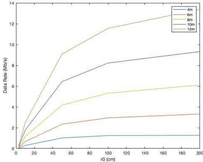
Figure 4. The achievable data rate for different effective  $r_0$  values. The lines correspond to a variety of telescope diameters.
