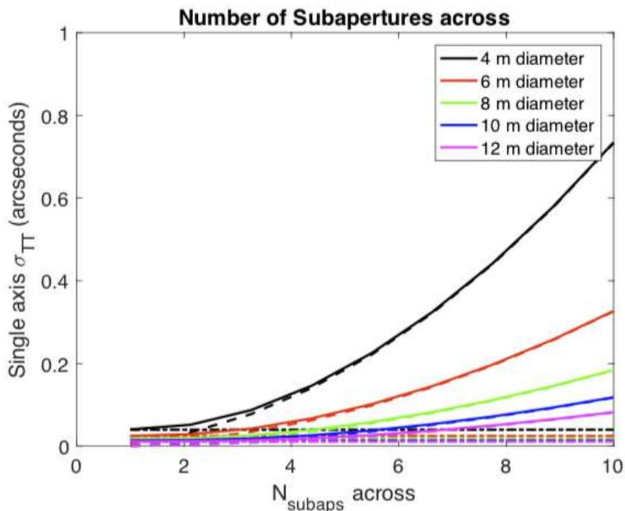
Figure 1. The tip/tilt measurement error in one axis as a function of the number of sub apertures across the primary aperture.
