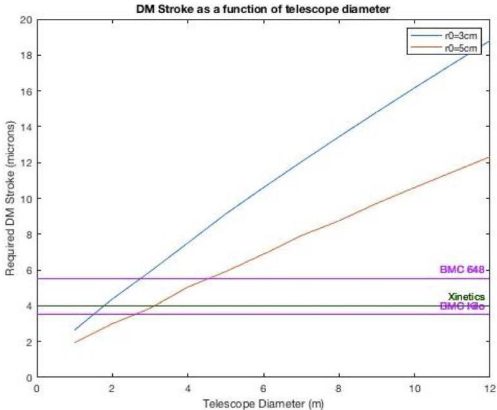
Figure 6. The required DM stroke required as a function of telescope diameter for multiple  $r_0$  values. The horizontal lines are the achievable stroke for three different DMs. All Xinetics surface normal DMs achieve the same stroke.
