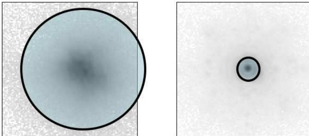
Figure 3. This figure shows the PSF for an uncorrected image on the left and an AO corrected image on the right. The black circles show the size of an aperture that would encompass most of the light of the PSF. AO enables the user to use a smaller aperture to capture the same amount of light with a dramatically reduced amount of background signal.
