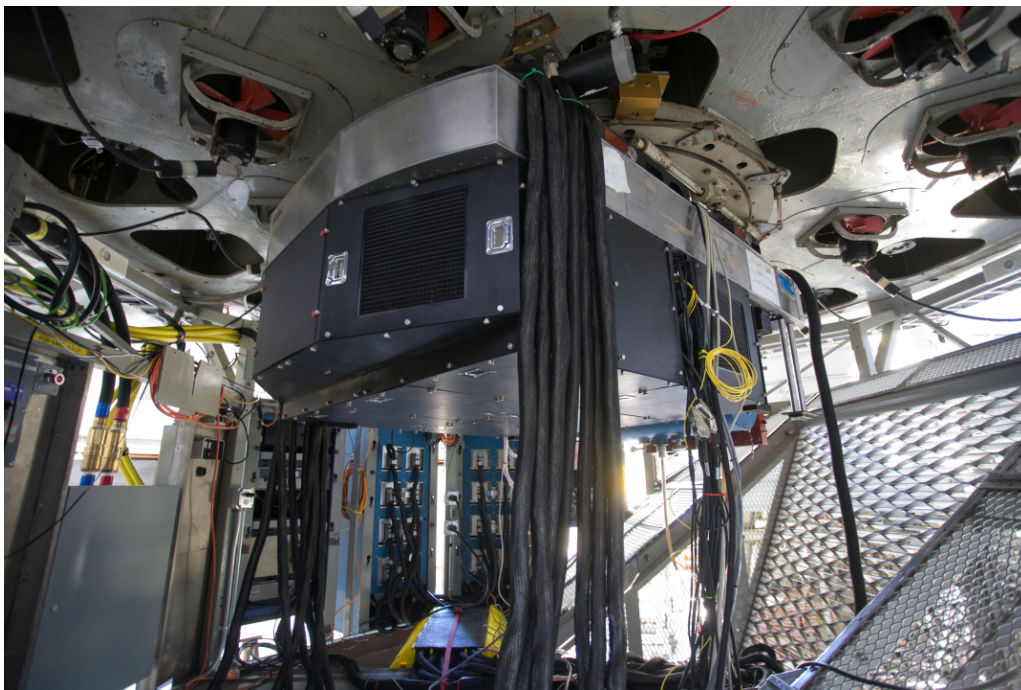
Figure 3 PALM-3000 installed at the Cassegrain focus of the Hale 200" telescope with the HODM cables in the foreground.
