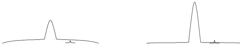
Figure 1. Adaptive optics corrected images of a faint companion in the presence of a bright astronomical source for (left) moderate Strehl ratio, and (right) high Strehl ratio.
